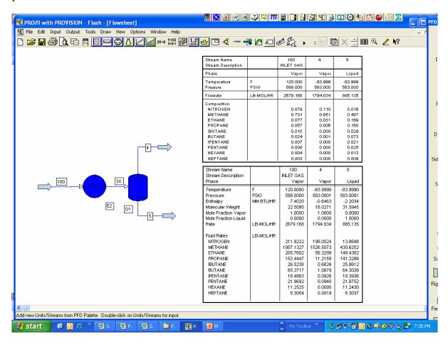
We notice that the liquids contain some methane so, we realize that a distillation column might be needed. However, we do not have a refrigerant to provide a reflux of methane. Therefore, we use a column without a condenser. To aid in the separation, we reduce the pressure in the column.
