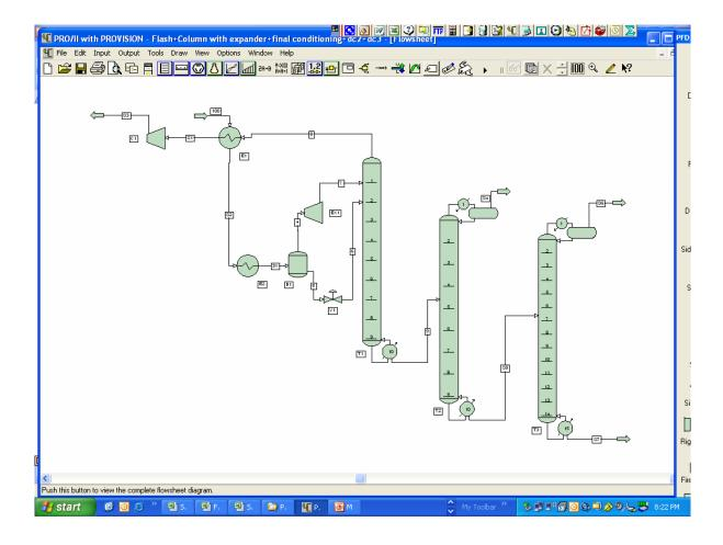
**EXERCISE 4-11:** Set up the simulation with a recovery of liquids as explained. Compare the possibility of recovering propane + butane instead of only propane.
